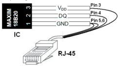
The cable of the detector can optionally be extended up to 50 meters with a network cable and a  $2\times RJ45$  adapter. (see pictures)
